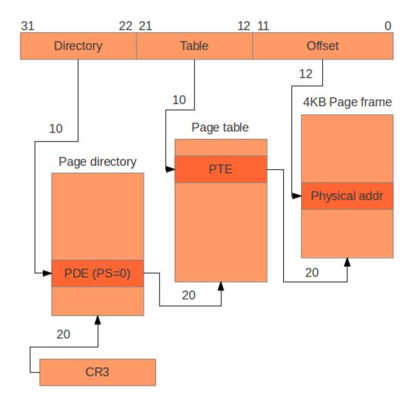
Figure 3: Translating virtual addresses (linear addresses) to physical addresses.
