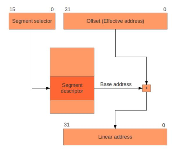
Figure 2: Translation of logical addresses to linear addresses.
